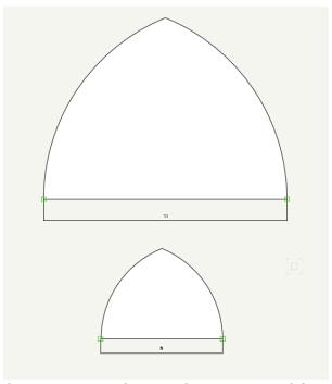
Begin the vault by drawing two arches. As this is a tutorial for a rectangular vault, our transverse arch and wall arch will be different sizes. This tutorial will use a 10 meter (diameter) quinto arch and a 5 meter quinto arch. However, your arches may be different (ex: quinto arch and tri arch, etc).
