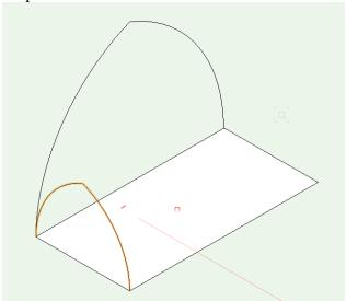
Rotate the smaller arch so that it is aligned with the shorter side of the rectangle. This may be easier to do in top view. When you switch back to right isometric, it will look like this.
