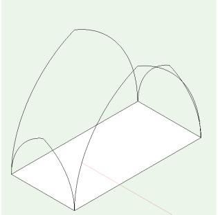
Select both arches and switch to top view. Select the mirror tool. Center the tool on the rectangle and mirror the two arches to the other side. You will now have an arch on each side of the rectangle.
