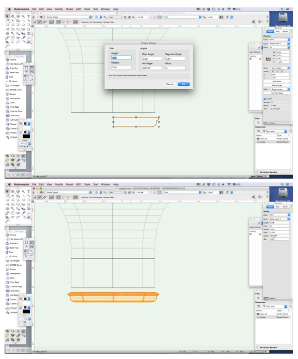
2. Position the astragal under the base of the capital. You will need to do this in top plan to assure proper alignment.
