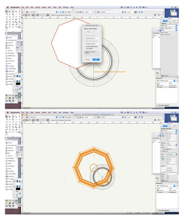
8. Now click and drag the object until it snaps to the center of the capital. \*Note: Check this looks correct in Right Isometric view before moving on. If it is incorrect, undo and retry Extrude Path making sure to check the "Fix Profile" in the popup window.
