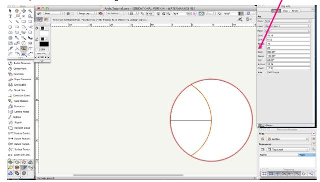
8. Now use the "Trim" tool to remove the segments below the horizontal line.
