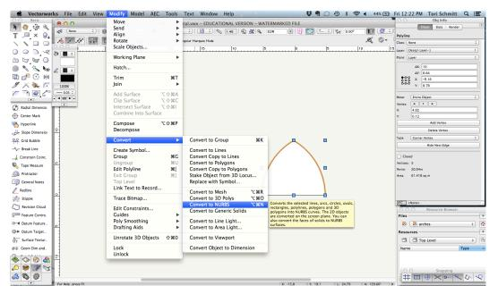
11. You may now delete the line you created in step 2 to indicate the arch span. We will now create the vertical sides of the arch. Select the "Line" tool from the "Basic Tools" palette and click at the left end of the NURBS Curve (Arch). Hit the tab key and enter 10m for the length of the line. Click to place the line.
