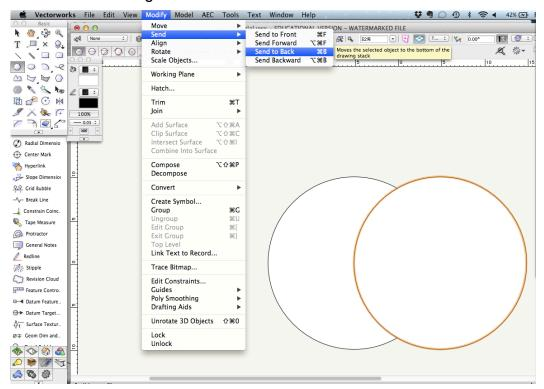
6. Select the "Trim" tool from the "Basic Tools" palette. Click on the outer ring of each circle to delete these segments. If you delete a portion unintentionally, hit "Command+Z" to undo.
