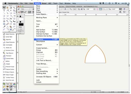
10. With the polyline selected, go to "Modify > Convert > Convert to NURBS." This will convert the shape from a polyline to NURBS. NURBS will allow the molding profiles to be extruded along a finished arch.
