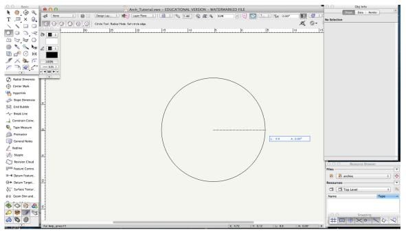
Select the "Circle" tool from the "Basic Tools" palette. Make sure the first mode (Radius Mode) is selected. Click to place the circle at the left end of the line. Extend the radius of the circle to the right end. The radius of the circle should be 10m
