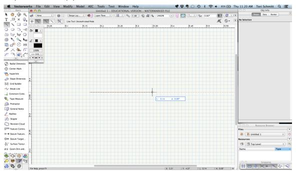
Select the Line tool from the "Basic Tools" palette. Click once to set the Line tool in the document. Hold the shift key and move the cursor to the right.
