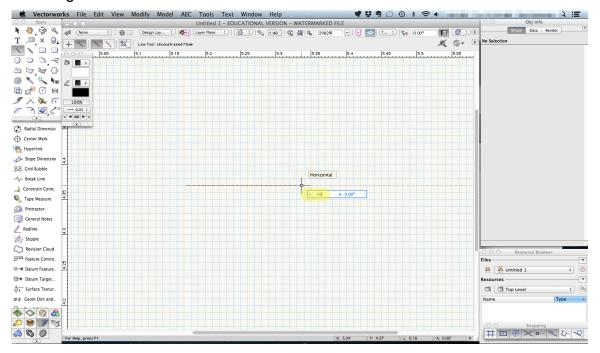
2. Hit the tab key to be able to enter 10m in the "L" field. Press enter. Click again to place the line. This step will ensure that the line is 10m in length.
